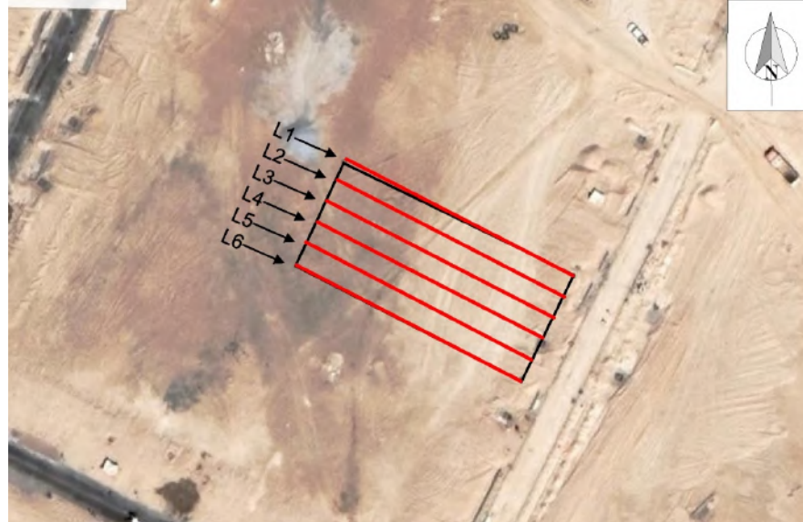
Figure 4: Seismic Lines design: (In Red the Final Sections location - Not in scale).
