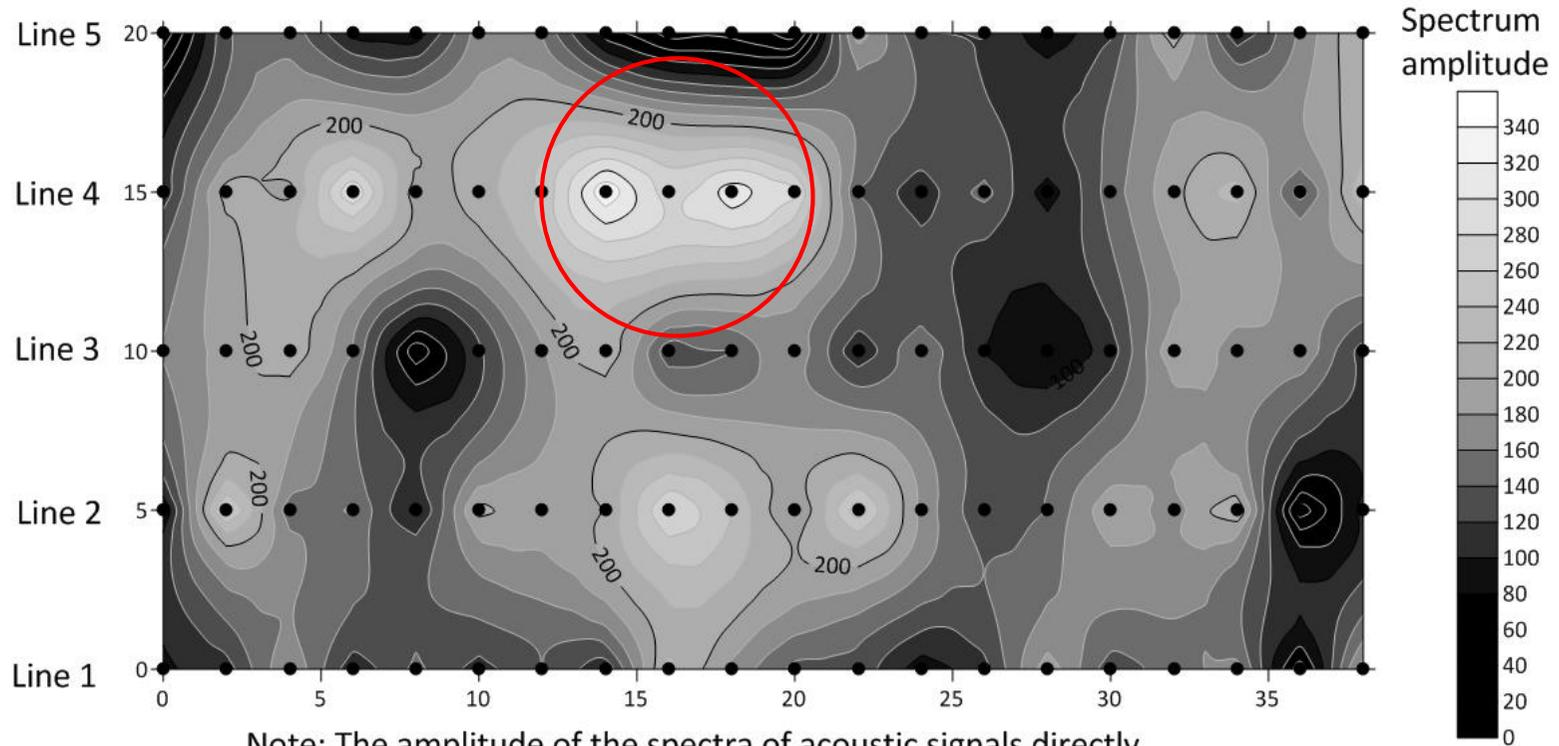
Note: The amplitude of the spectra of acoustic signals directly associated with the mechanical strength of the section rocks. The higher amplitude of the spectrum - the less mechanical strength of rocks (higher degree of fracturing, watering, etc.)
