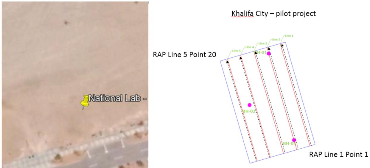
Figure 2. Satellite Image and surveyed geophysical lines for both MASW and RAP lines
