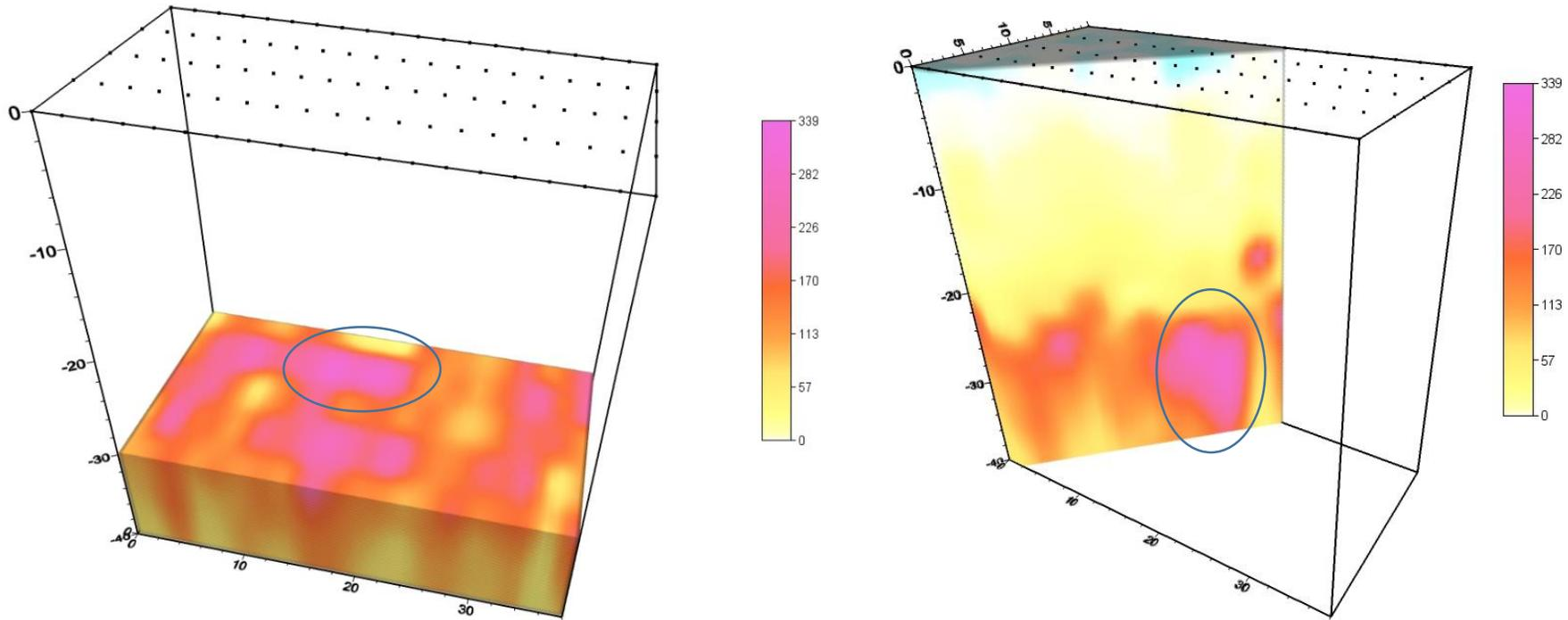
**Significant anomaly appears as very weak zone at 30+ meters depth at the 16-meter mark (Point 9) of Line 4**
