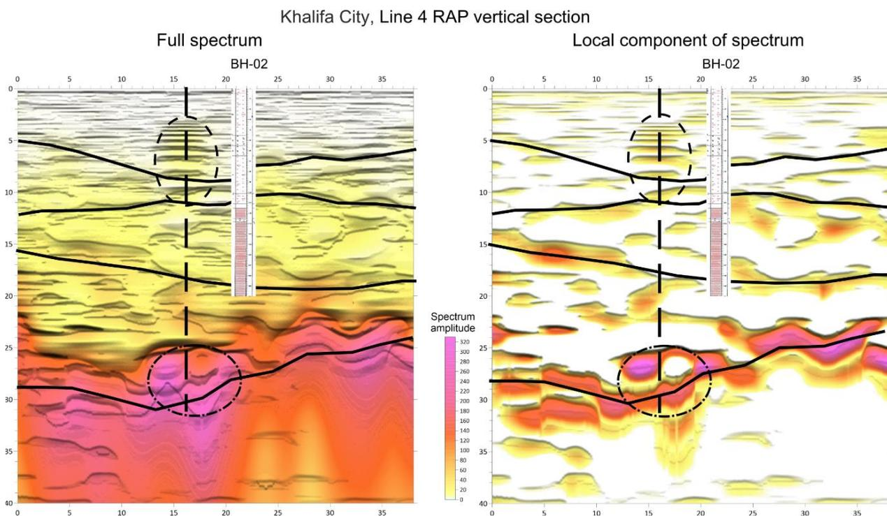
**Figure 5. 2-D RAP profile obtained from survey Line 4; full spectrum at left and local component at right**
