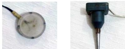
**Figure 6. Two types of piezoelectric sensors available for use with RAP: flat sensor on the left and sensor with spike on the right. Flat sensor can also be placed on top of a steel spike in certain conditions.**
