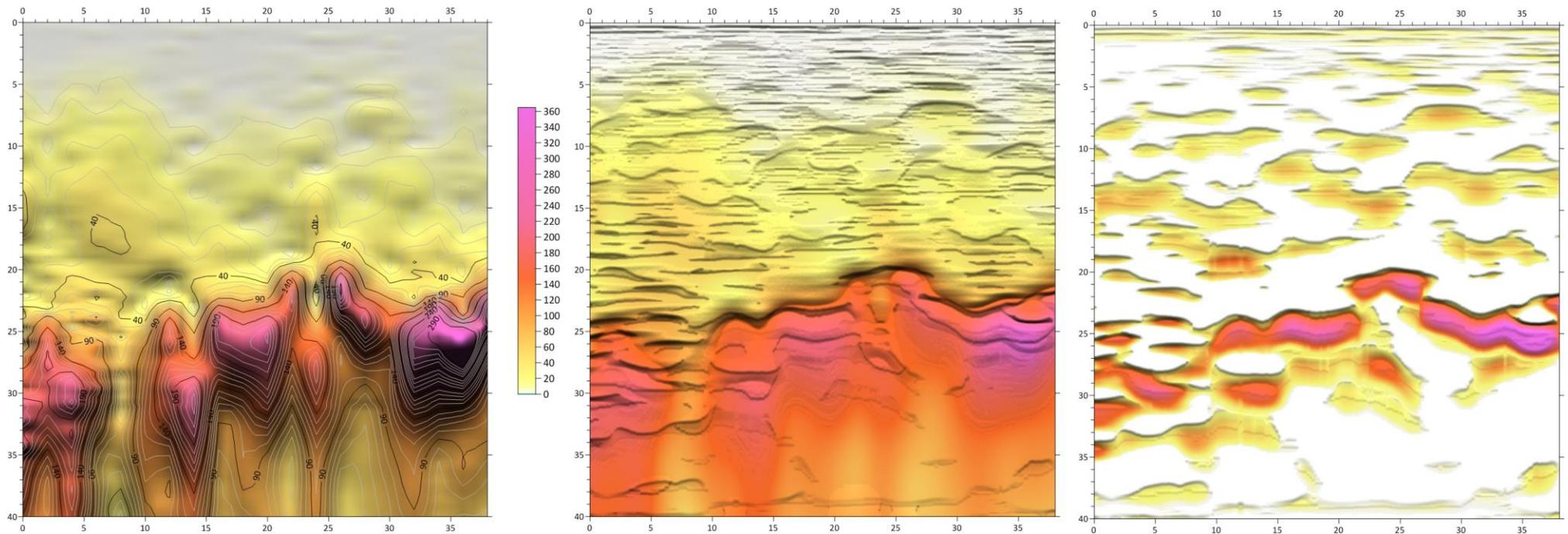
***The profile on the left presents the Full Spectrum as visualized in Surfer with relief map overlaying contour map. The second profile is Full Spectrum processed and visualized in Centre program. The third profile is a presentation of the Local Component of the Spectrum, also processed and visualized in Centre program.***
