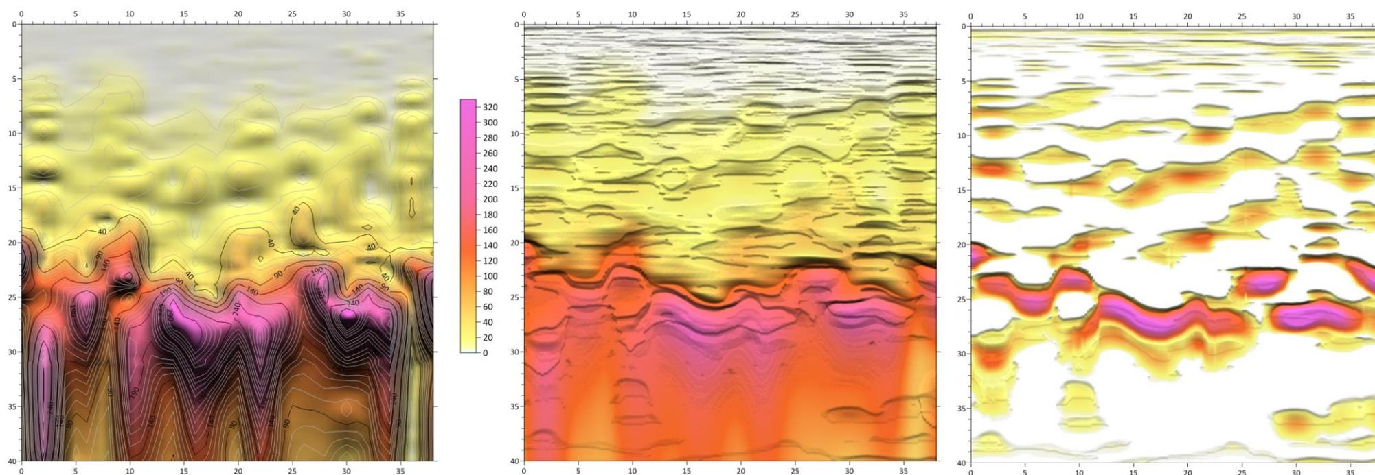
***The profile on the left presents the Full Spectrum as visualized in Surfer with relief map overlaying contour map. The second profile is Full Spectrum processed and visualized in Centre program. The third profile is a presentation of the Local Component of the Spectrum, also processed and visualized in Centre program.***
